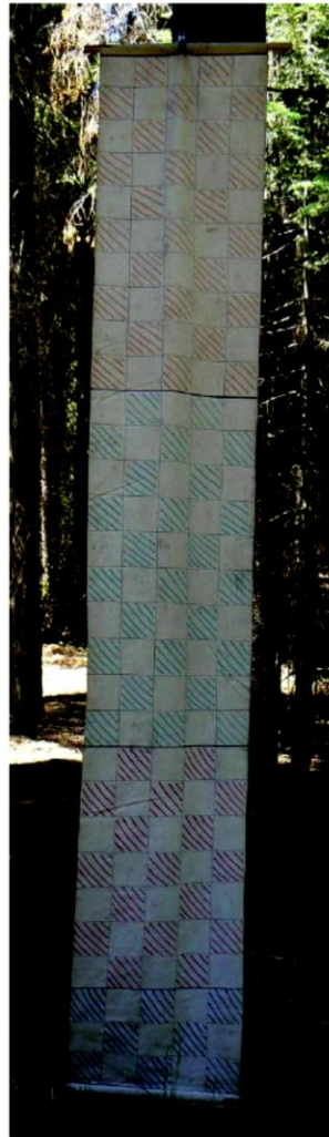
Figure A5. Design and use of coverboard for estimating concealment cover around the base of den trees. The coverboard is divided into four sections representing low ground cover, high ground cover, low shrub cover, and high shrub/small tree cover.
